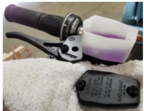
Figure 1. Cap removed from master cylinder reservoir
