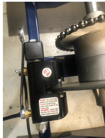
Figure 3. Dual caliper brake system
