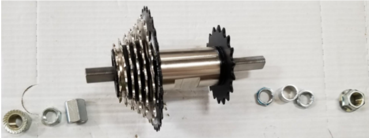
Figure 9. Transfer hub should use on freewheel side an outer jam nut, and then a wide nut up against bearing. The rear cog side will have an outer jam nut, spacer and inner jam nut against bearing.
