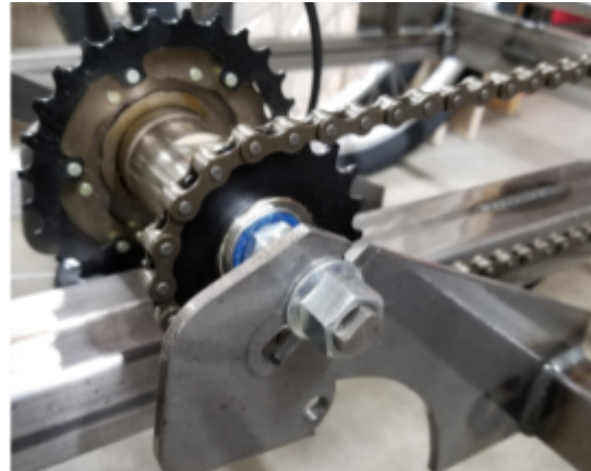
Figure 12. Transfer hub positioned halfway down dropouts
