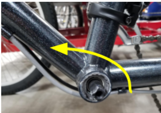
Left side of bottom bracket - turn counterclockwise to remove
