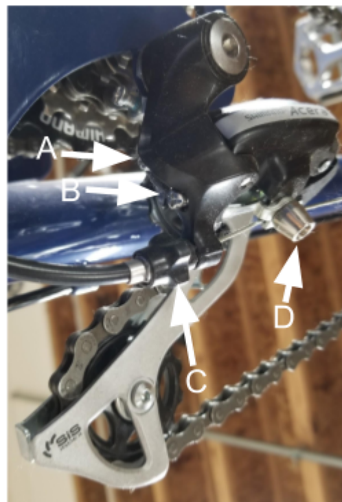
Figure 8. Rear derailleur. A) High limit screw; B) Low limit screw; C) Barrel Adjuster; D) 5 mm cable bolt
