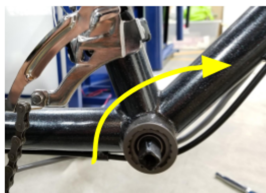
Right (drive) side of bottom bracket - turn clockwise to remove
