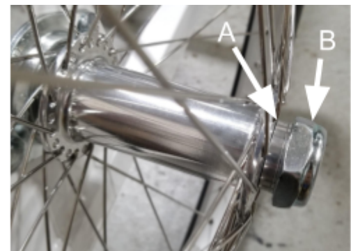
Figure 15. Rear wheel hub and axle nut assembly. A) Axle spacer; B) Axle nut
