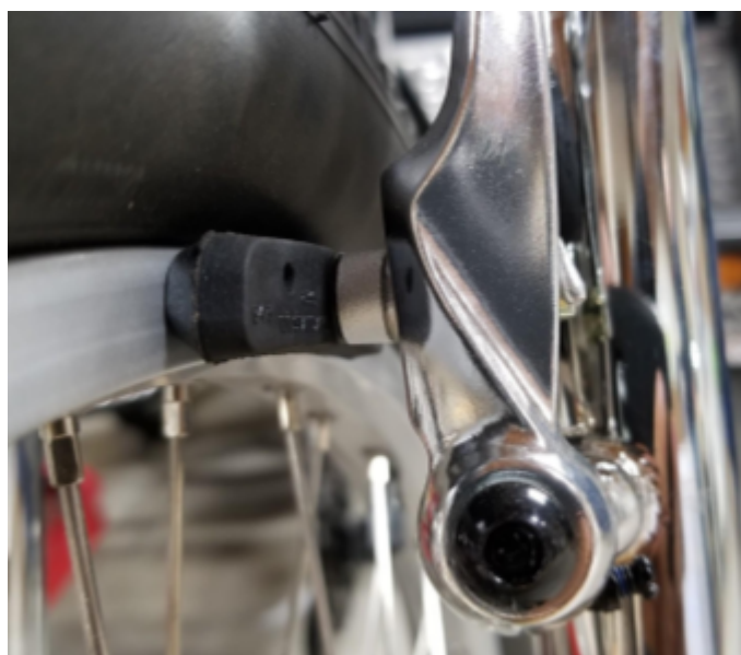
Figure 6. Correct brake pad positioning
