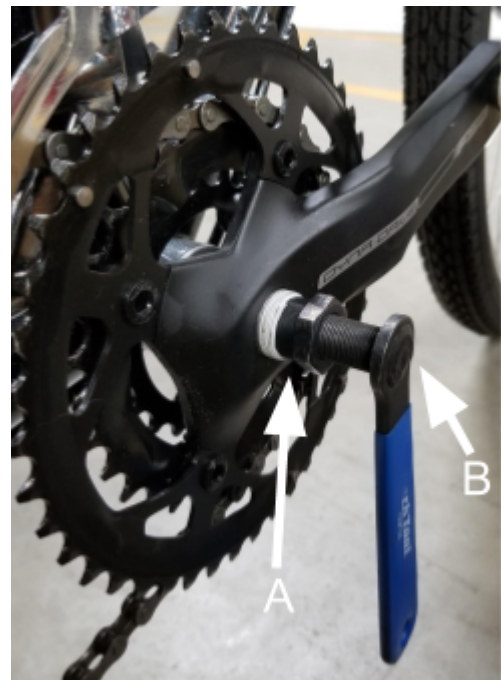
Figure 14. Crank puller installed. A) Puller Nut; B) Spindle driver
