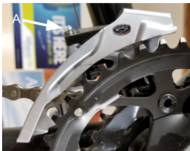
Figure 7. Front derailleur positioning; A) limit screws
