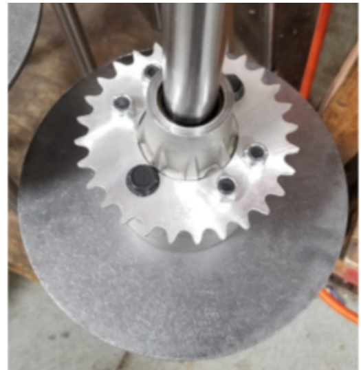
Figure 16. Sprocket side of differential - showing two bolts going into housing and four nuts on bolts all the way through housing
